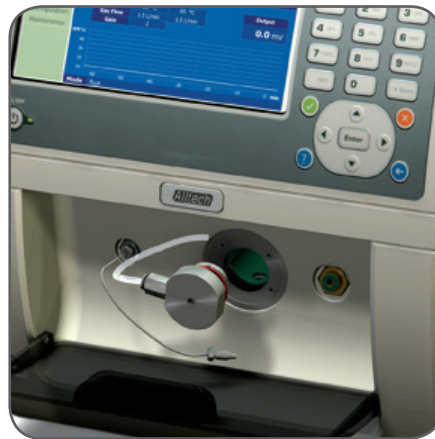
Remove the nebulizer with a simple twist and pull
